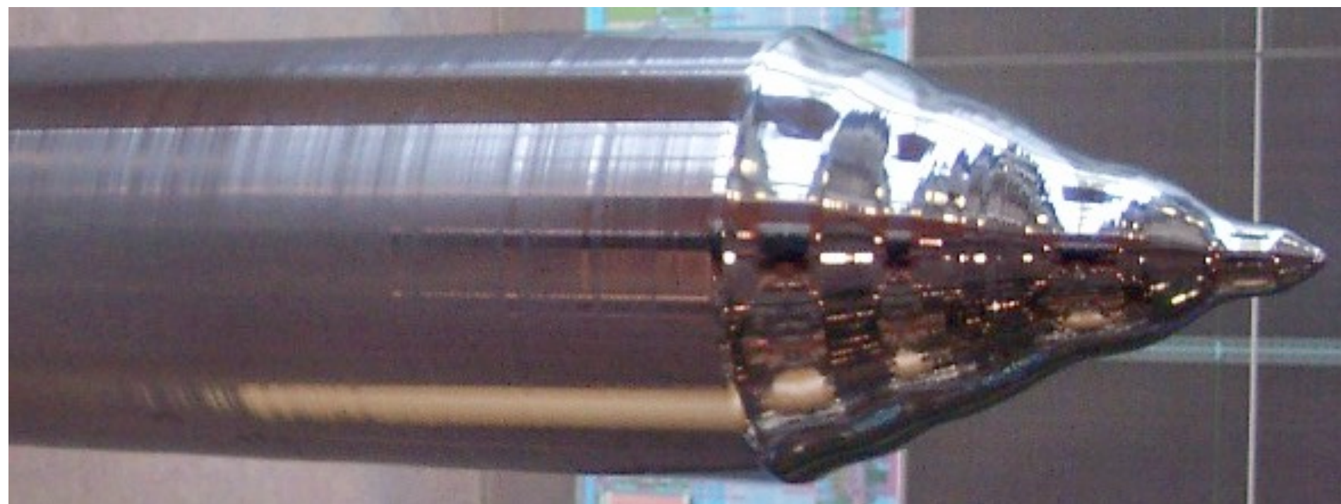
A silicon boule, as grown
